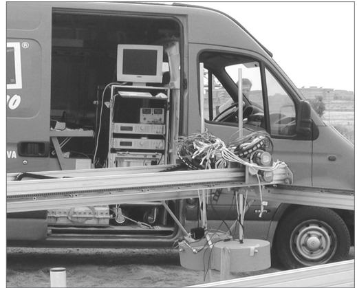
Fig. 1. The rack of the GPR inside the van during data acquisition campaign.
