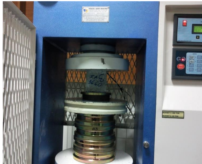
Fig. 2. Compressive strength test
