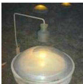
Fig. 13. Artificial light above the Conical skylight
