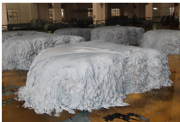
Fig. 1. High quality bovine wet blue manufacture: High volume manufacture using closed-loop technology.
