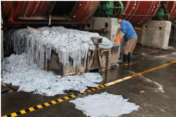
Samples showing wet blue sheep skin leathers. Float recovery at the rear of the drum row before filtration and storage.
