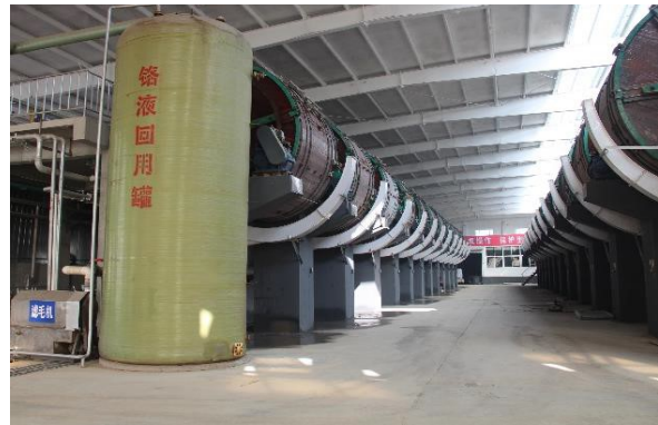
Shows an isolated liming zone in a new-build tannery complete with holding tank.
