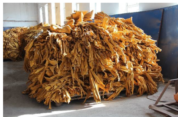
Full hide manufacture is limited by the width of the fleshing machine, hence specialist belly leather processing. Air dried/tension free, these leathers are ideal for bags and leather goods.
