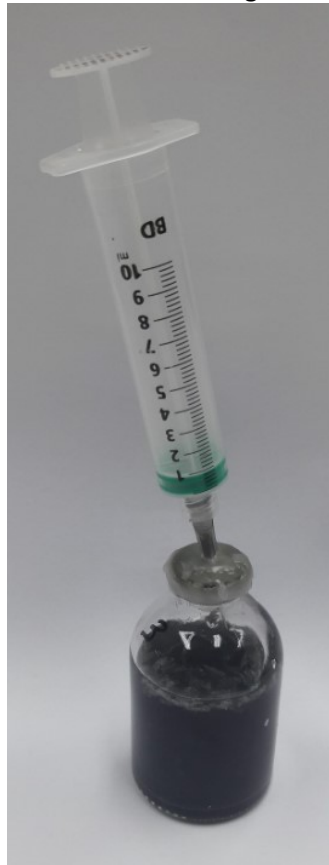
Fig 1. Biodegradation test in 50 mL flask with monitoring of biogas production with graduated syringe.
