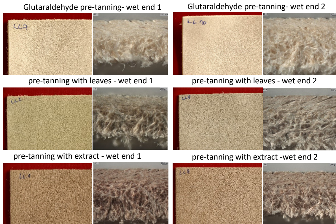
Figure 10. Photos and microscopic images (50x) of leathers of tanning agents from privet leaves and glutaraldehyde.
