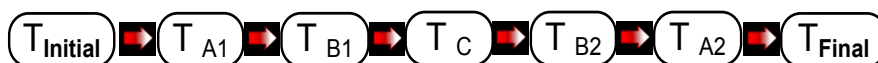
Fig. 1. Temperatures defining each step according to fibers shrinkage: T_{\text{Initial}} (the material fibers are inactive), A1 (the first shrinkage of individual fibers is noticed), B1 (the individual fiber shrinkage is immediately followed by another fiber shrinkage consecutively), C (most fibers experience simultaneous shrinkage), B2 (the last fibers experience simultaneous shrinkage), A2 (the shrinkage of the last individual fibers is noticed), T_{\text{Final}} (fibers shrinkage is complete).
