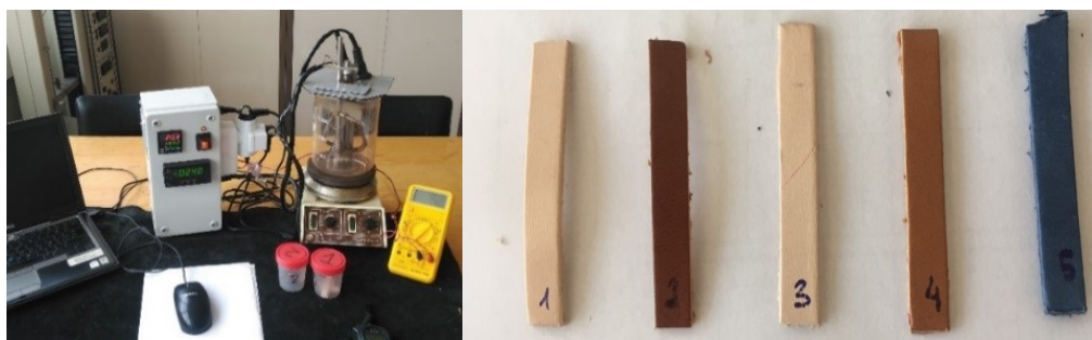
Fig. 3. Experimental device used to measure T_s and tanned leather probes.
