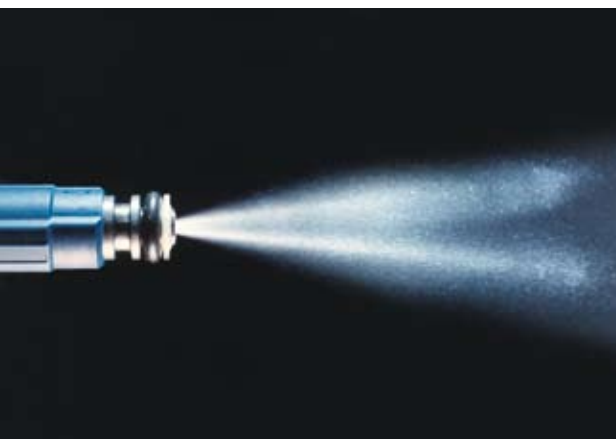
The jet from an injector nozzle for the Bosch DI-Motronic gasoline direct injection system (2005).
