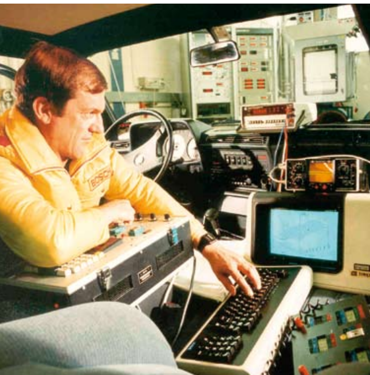
Left: Testing “Motronic” at the Automotive Engineering Center in Schwieberdingen, near Stuttgart (1984). In 1979, the Motronic installed in the BMW 732i was the first system to manage injection and ignition from a single control unit.
