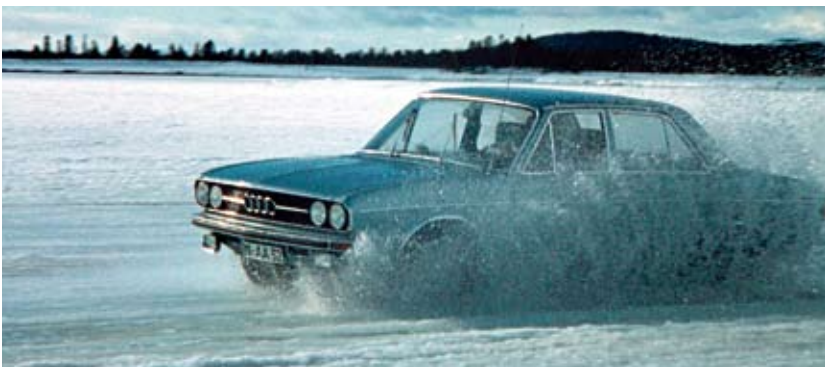
In Arjeplog, northern Sweden, Bosch tests chassis systems on frozen lakes. The picture shows an Audi 100 GL featuring a pilot version of ABS (1975).
