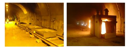
Fig.1. Fire pools on rail tracks used for heating the concrete surface of the Minitunnel (right picture)
