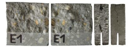
Fig. 5: Example of fracture surface and crack path for selected specimen E1
