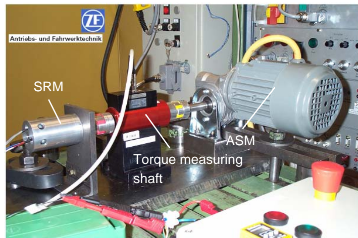
Fig. 6.19 Test bench with SRM III in the laboratory of the ZF Friedrichshafen AG
