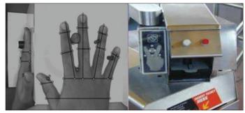
**Figure 5:** Hand and two finger geometry measurements. Source: Ross et al., n.d
