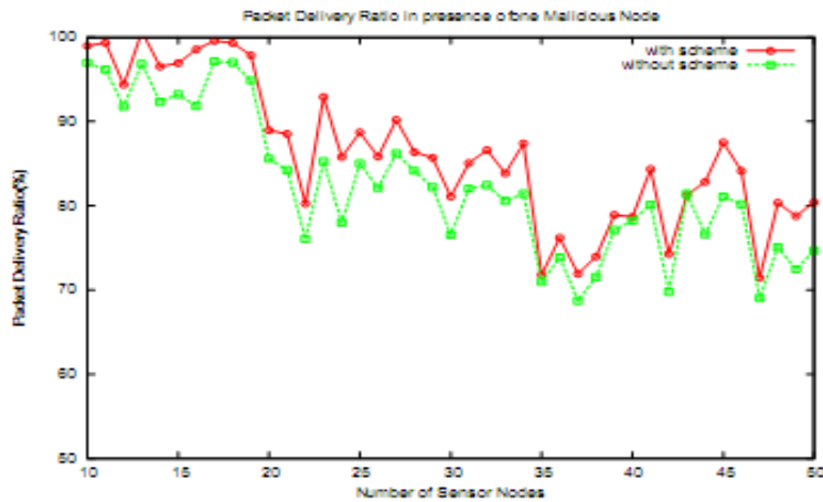
Figure 5: Packet Delivery Ratio vs. Number of Sensor Nodes in the presence of one Malicious Node
