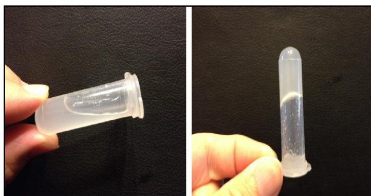
FIGURE 4: Development of in vitro hydrogel with in situ gels and artificial tear fluid using gellan gum as polymer adapted from Lina Zhu et al.,(2015).
