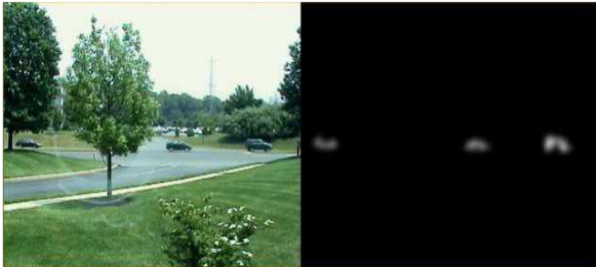
Fig.3. Detection for a traffic sequence consisting waving tree using kernel density estimation
