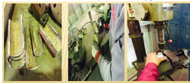
Figure 3: Cutting process of carbon steel samples
