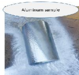
Figure 8: carbon steel pipe sample coated with aluminum.
