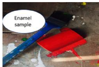
Figure 10: carbon steel pipe sample coated with Enamel.
