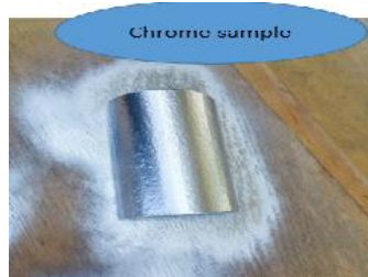
Figure 7: carbon steel pipe sample coated with chrome.
