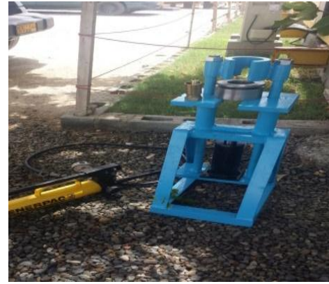
Figure 4 Final assembly of the crimping machine
