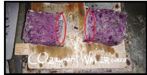
Fig. 5. CO 2 Cured and Water Cured Concrete Cubes
