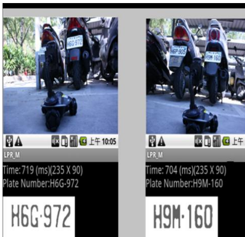
Figure 9. Field trial about OCR results of Android-based robot featuring LPP and LPR.
