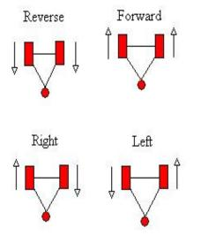
Fig 1. Movement of the Robot
