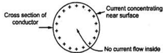
Figure 1 Cross section view of conductor on skin effect
