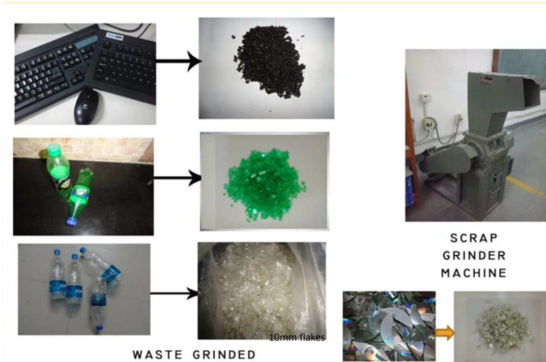
Figure 1: The scrap grinder machine and the grinded material from the base material
