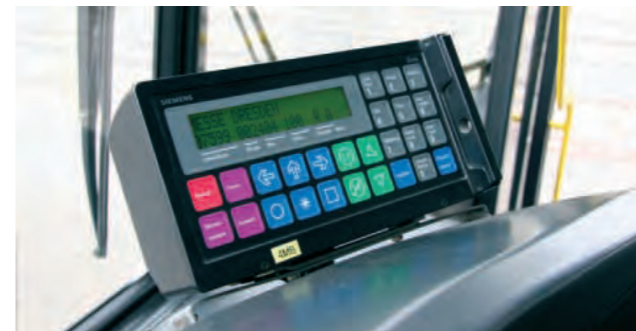
More information for the driver: On-board computers in the driver's cab of trams and busses are constantly updated.
