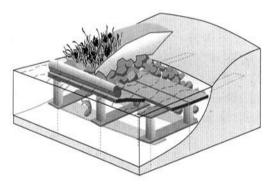
Cells constructed of heavy wooden planks and blocks which are imbedded into the toe of streambanks at channel bed level to provide covered compartments for fish shelter, habitat, and prevention of streambank erosion.
