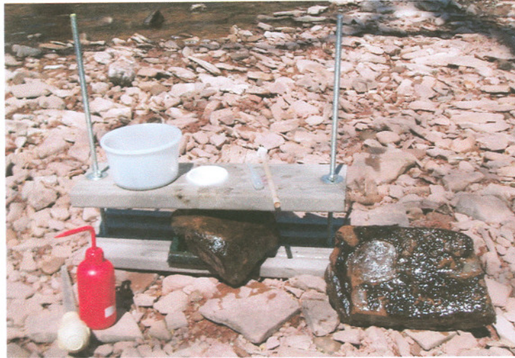
Figure 2. Photo of PEP sampler designed by PADEP (Photo provided by Alan Everett, PADEP)
