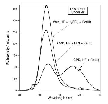
Figure 3. Etching >8 h leads to a significant blueshift in the PL. In the absence of added HCl or  $H_2SO_4$ , the development of the peak near 530 nm was significantly slower. The samples were etched for 17.5 h with 1.65 g of FeCl<sub>3</sub>·6H<sub>2</sub>O added to 10 mL HF or 1 mL HCl + 9 mL HF or 1 mL  $H_2SO_4$  + 9 mL HF.
