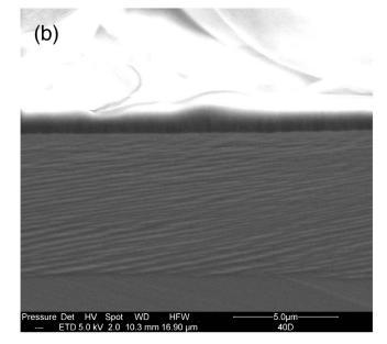
**Figure 1.** Two cross-sectional SEM images from porous silicon. Etching in 1.37 g FeCl<sub>3</sub>·6H<sub>2</sub>O + 3 mL H<sub>2</sub>SO<sub>4</sub> + 7 mL HF for 22.5 h, under Ar; rinsing in water and methanol; and drying in a stream of Ar led to exfoliation and destruction of the upper part of the film. (a) The exfoliated region exceeded 5  $\mu$ m in thickness, whereas (b) the film that remained intact and attached to the substrate exceeded 6  $\mu$ m in thickness.
