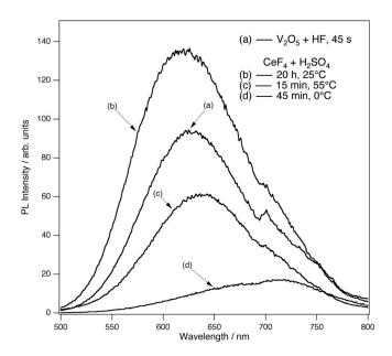
**Figure 4.** The PL spectra of (a) a film etched for 45 s in a V-based etchant containing 0.25 g  $V_2O_5$  in 10 mL HF; (b–d) samples produced in the Cebased etchant made from a saturated solution of CeF<sub>4</sub> dissolved in (5 mL H<sub>2</sub>SO<sub>4</sub> + 5 mL H<sub>2</sub>O), (b) etched 20 h at 25°C, (c) etched 15 min at 55°C, and (d) etched 45 min at 0°C.
