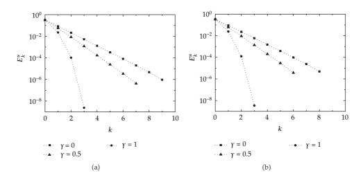
**Figure 1:** The error  $E_k^u$  with respect to *k* for each method (fixed point:  $\gamma = 0$ , hybrid:  $\gamma = 0.5$ , Newton:  $\gamma = 1$ ). The error  $E_k^u$  obtained with the coarsest mesh is displayed on (a) and the error  $E_k^u$  obtained with the finest mesh is displayed on (b).
