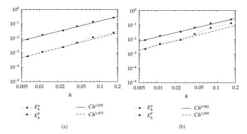
**Figure 2:** The errors  $E_h^u$  and  $E_h^p$  with respect to *h* with  $\theta = 2$  (a) and with  $\theta = 1.34$  (b). Regression straight lines have been drawn from the last three points of each set of six recorded errors.
