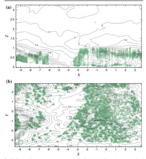
Fig. 11 Skewness of the mean streamwise velocity component fluctuations  $S_u$ . The coordinates are normalized according to Eqs. 10. Skewness is calculated from instantaneous snapshots following Eq. 14. Colouring depicts the *PAD* values. **a** Vertical slice at Y = 0. **b** Horizontal slice at Z = 0.8
