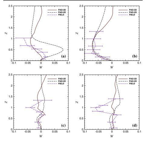
**Fig. 8** Comparison of measured and computed normalized vertical velocity profiles at the four measurement towers. The normalization is according to Eqs. 10 and 11. The tower positions are given in Fig. 1. **a** Tower T1, **b** Tower T2, **c** Tower T3, **d** Tower T4
