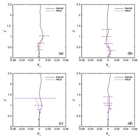
**Fig. 14** Comparison of measured and computed profiles for normalized Reynolds stress  $R_{yz}$  at the four measurement towers. The normalization is according to Eqs. 10 and 12. The tower positions are given in Fig. 1. **a** Tower T1, **b** Tower T2, **c** Tower T3, **d** Tower T4
