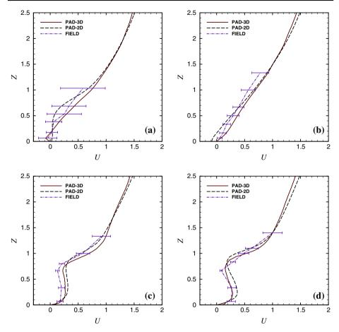
**Fig. 7** Comparison of measured and computed normalized streamwise velocity profiles at the four measurement towers. The normalization is according to Eqs. 10 and 11. The tower positions are given in Fig. 1. **a** Tower T1, **b** Tower T2, **c** Tower T3, **d** Tower T4
