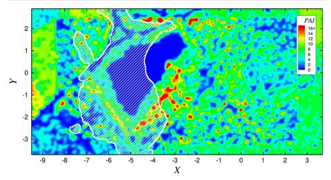
Fig. 6 Projected horizontal contours of the separation zone. Colouring depicts the *PAI* values with  $2 \text{ m} \times 2 \text{ m}$  filter width
