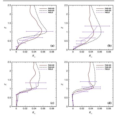
Fig. 13 Comparison of measured and computed profiles for normalized Reynolds stress  $R_{XZ}$  at the four measurement towers. The normalization is according to Eqs. 10 and 12. The tower positions are given in Fig. 1. **a** Tower T1, **b** Tower T2, **c** Tower T3, **d** Tower T4
