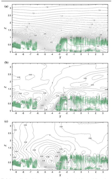
**Fig. 3** Contours of the dimensionless mean velocity components for a vertical slice at Y = 0. The coordinates and values are normalized according to Eqs. 10 and 11. Colouring depicts the *PAD* values. **a** U, **b** V, **c** W
