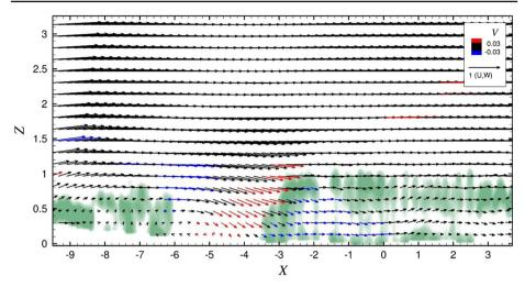
**Fig. 4** Dimensionless mean velocity vector (U, V, W) in the plane Y = 0. Colouring of the vector depicts the lateral velocity component (V), with *red* indicating positive (northward) and *blue* negative (southward) motion. The coordinates and values are normalized according to Eqs. 10 and 11. The *empty area* in the *lower left corner* contains no data as it is located below the surface level. *Background colouring* depicts the *PAD* values
