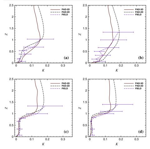
**Fig. 12** Comparison of measured and computed profiles for normalized turbulent kinetic energy K at the four measurement towers. The normalization is according to Eqs. 10 and 13. The tower positions are given in Fig. 1. **a** Tower T1, **b** Tower T2, **c** Tower T3, **d** Tower T4
