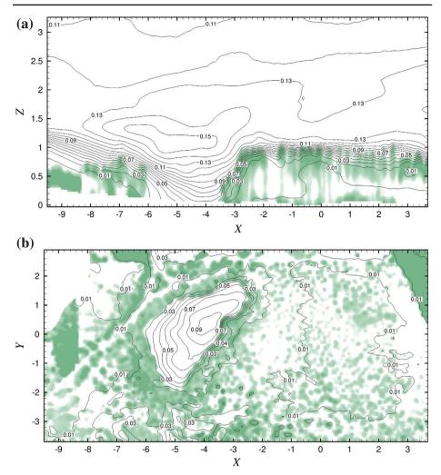
**Fig. 9** Normalized turbulent kinetic energy *K*. The coordinates and values are normalized according to Eqs. 10 and 13. Colouring depicts the *PAD* values. **a** Vertical slice at Y = 0. **b** Horizontal slice at Z = 0.3
