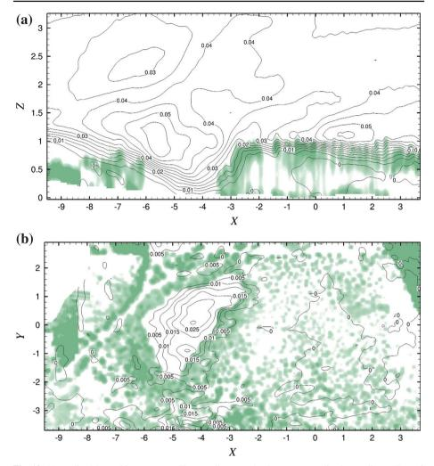
Fig. 10 Normalized Reynolds stress  $R_{XZ}$ . The coordinates and values are normalized according to Eqs. 10 and 12. Colouring depicts the *PAD* values. **a** Vertical slice at Y = 0. **b** Horizontal slice at Z = 0.3
