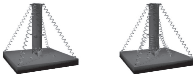
Figure 3: Illustration of a model with four large springs (left) and another model with four large and four strong small springs. The model works with the assumption that the small springs can sense a change in movement faster than the large springs. (Form Nigg, 2005, with permission).
