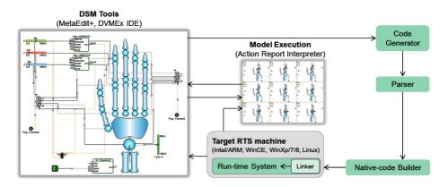
Figure 8. Platform for model execution and model-level debugging
