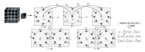
Figure 2. Illustration of our method to extract PDVs from a volume both spatially and temporally. Here we just show the process of calculating the frames at time  $t - \Delta t$  and  $t + \Delta t$  to current frame at time t. The same process can be used for depth data after computing the gradient of each frame.
