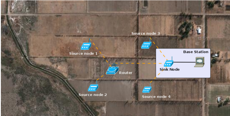
Figure 2. WSN for frost prediction in Mendoza, Argentina
