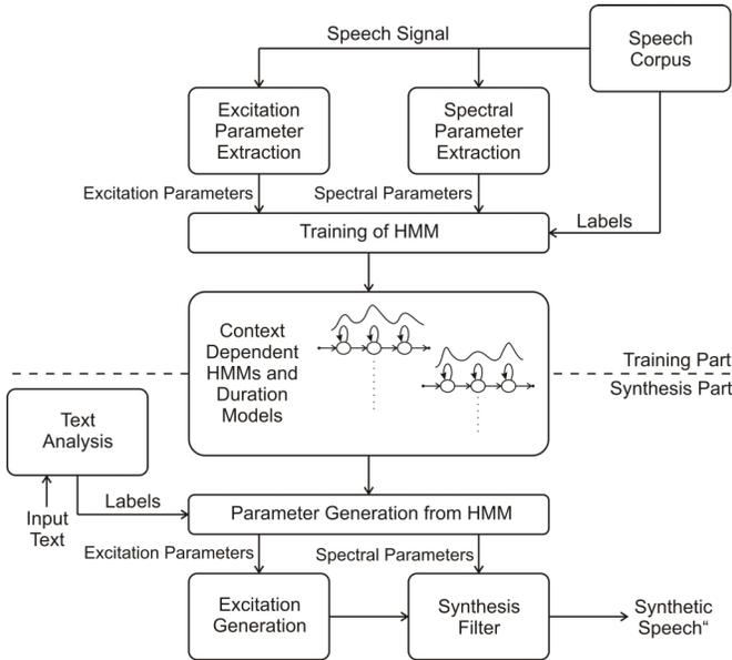
Figure 1. Block diagram of the HMM-based speech synthesis system
