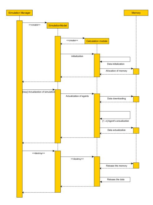
Figure 1. Sequence diagram of presented application
