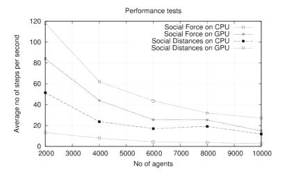
Figure 3. Results of performance tests for social force and social distances models implemented respectively on CPU and GPU
