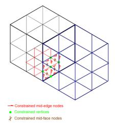
Figure 2. The breaking of large element followed by breaking of one of the small elements
