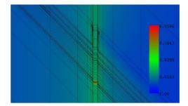
Figure 23. Exemplary resulting potential at the receiver electrode for a single position of a logging tool for 60 degrees deviated well
