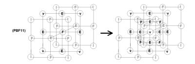
Figure 11. Graph grammar production (**PBF11**) enforcing breaking of a face surrounded by two interiors broken in two directions
