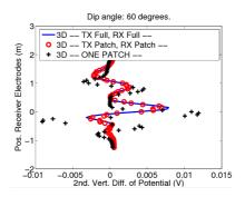
Figure 25. Logging curve for different antennas for 60 degrees deviated well case
