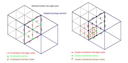
Figure 1. Left panel: Two adjacent elements, one broken into eight son elements. Right panel: The forbidden state with double constrained nodes.
