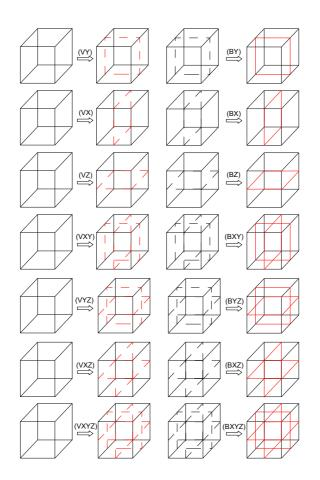
Figure 13. Graph grammar production for anisotropic breaking of a single element
