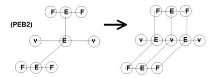
Figure 12. Graph grammar production (**PEB2**) enforcing breaking of an edge surrounded by two broken faces
