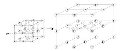
Figure 7. Graph grammar production (VXY) for virtual refinement of a single element into X and Y directions
