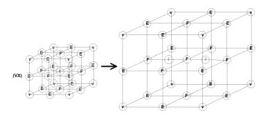
Figure 6. Graph grammar production (VX) for virtual refinement of a single element into X direction
