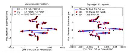
Figure 24. Left panel: Logging curves for different antennas for axial-symmetric case. Right panel: Logging curve for different antennas for 30 degrees deviated well case.
