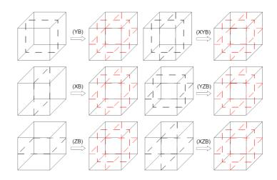
Figure 18. Additional graph grammar productions for removing of the dead-end problem
