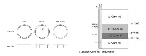
Figure 21. Left panel: The geometry of antennas. Right panel: The conductivities of the borehole, mandrel and formation layers in cylindrical coordinates.
