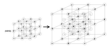
Figure 8. Graph grammar production (VXYZ) for virtual refinement of a single element into X, Y and Z directions
