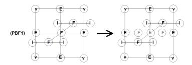
Figure 9. Graph grammar production (**PBF1**) enforcing breaking of a face surrounded by two interiors broken in one direction
