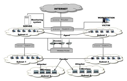
Figure 5. TUIDS testbed: All TUIDS datasets are prepared using this testbed with a number of configurations for the network as well as capturing tools
