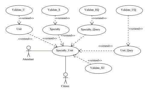
Fig. 4. UML use cases diagram of a considered part of the Health-Watcher system
