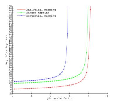
Fig. 17. Latencies provided by different mappings for a  $10 \times 4$  mesh
