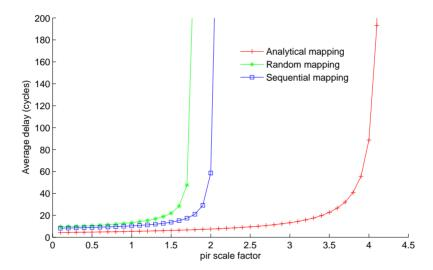
Fig. 21. Latencies provided by different mappings for the shuffle traffic distribution
