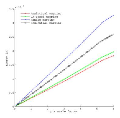
Fig. 16. Energy consumption required by the mapping techniques
