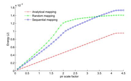
Fig. 22. Energy consumption required by different mappings for the shuffle traffic distribution
