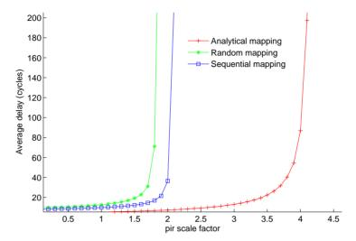
Fig. 19. Latencies provided by different mappings for the bit-reversal traffic distribution
