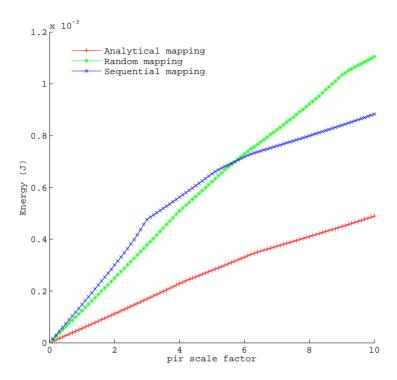
Fig. 18. Energy consumption required by different mappings for a  $10 \times 4$  mesh
