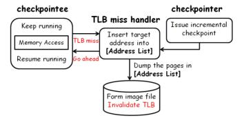
Fig. 3. Incremental checkpointing algorithm
