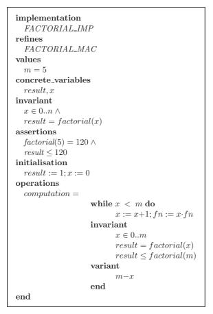
Fig. 13. An example of an implementation for the factorial computation
