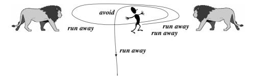
Fig. 11. An example of fluidity: The system in Figure 10 is not able to escape from the presented situation as it is attacked by two lions. In this case the *run away* command turns it still back – from one lion to the other. However, the *obstacle* agent, which tends to turn the system to the left, can help here although it is not responsible for getting away from lions. This is possible because both agents are still active. An agent cannot be passive, only its activity can have no effect
