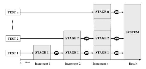
Fig. 13. Incremental development by subsumption
