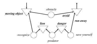
Fig. 10. An example of a fast but not sound reaction later improved: when a lion is met, the system at first tries to avoid it as an obstacle, only later the lion is recognized as a dangerous predator and the system tries to escape
