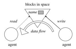
Fig. 1. A dataflow between two agents provided by space
