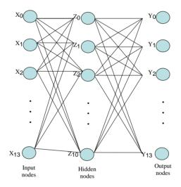
Fig. 1. MLP and RBF architecture used in the experiment
