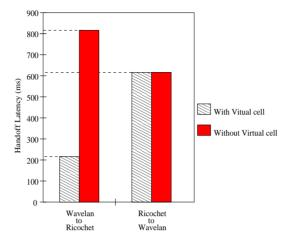
Fig. 10. Vertical handoff latency with beacon period of 200 ms
