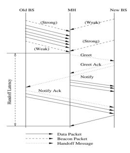
Fig. 2. Breakdown of horizontal handoff
