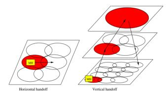
Fig. 1. Horizontal vs. vertical handoffs
