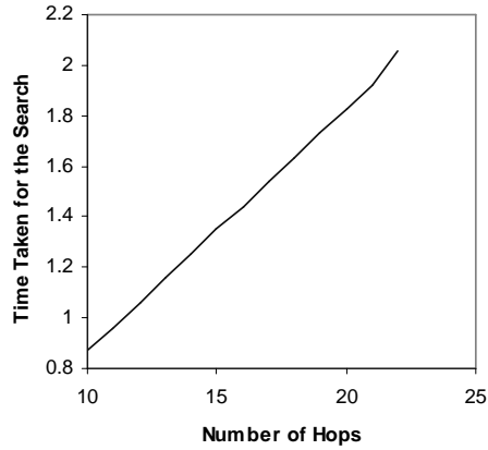
Fig. 10. Effect of number of pull MA hops on service time
