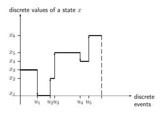
Fig. 1. The development of the state in the simple example of DEDS
