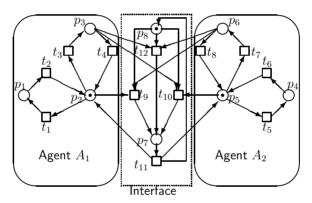
Fig. 18. The example of the PN-based model of the two agents communication in general
