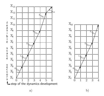
Fig. 11. The cooperation of two agents A1, A2 in MAS: a) the case when A1 solves (on the basis of the demand of A2) the problem to be solved by A2, however, A2 is not able to do this; b) the case when A1 refuses to help A2
