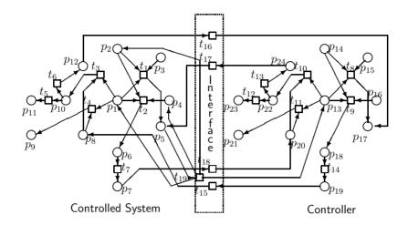
Fig. 14. The PN-based model of the feedback cooperation of the  $A_{syst}$  and  $A_{cont}$
