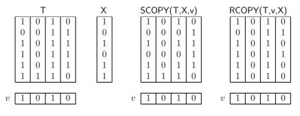
Fig. 1. The use of SCOPY(T, X, v) and RCOPY(T, v, X)
