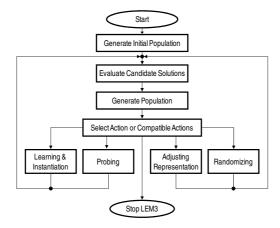
Fig. 1. Flowchart of the top level LEM3 algorithm
