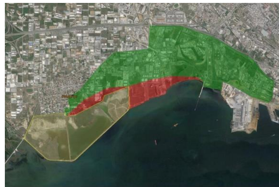
Figure 3.10 : Settlements at potentially liquefiable areas for p=100\text{kPa} ( a=0.25g - M=6.5\text{Richter} )
