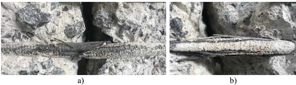
Fig. 3.19. Failure modes of basalt fibre reinforced polymer bars at the failure crack a) bending failure b) broom-shape tension failure
