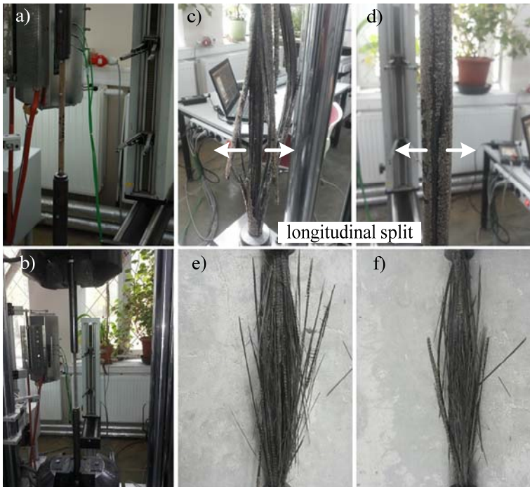
Fig. 3.5. Basalt Fibre Reinforced polymer specimen: a)-b) before fatigue test; c)-d) failure mode by longitudinal split; e)-f) broom-shape failure pattern
