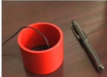
Fig. S1.1. a prototype of the cylinder-type piezoactuator (Bansevicius 2007).
