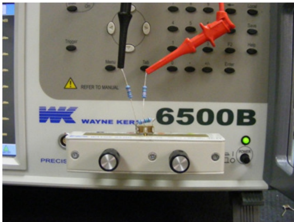
Fig. 4.2. Outside view of capacitor test setup
